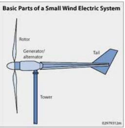
As wind moves over the turbine blades, it creates high-pressure air below the turbine blades and low-pressure air above them, causing 'lift', just like an airplane.
