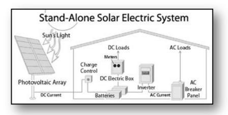
**Stand Alone Power** systems rely exclusively on solar energy to meet a need for electricity. As mentioned in the preceding, they may incorporate batteries which store energy from the PV modules during the day – for use at night or in periods of low solar radiation.
