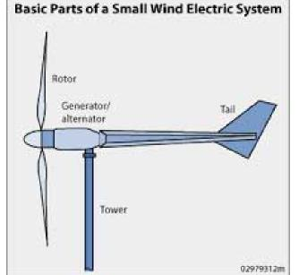
A generator produces Direct Current (DC) power or an alternator produces Alternating Current (AC) power, depending on what type of turbine you have.
