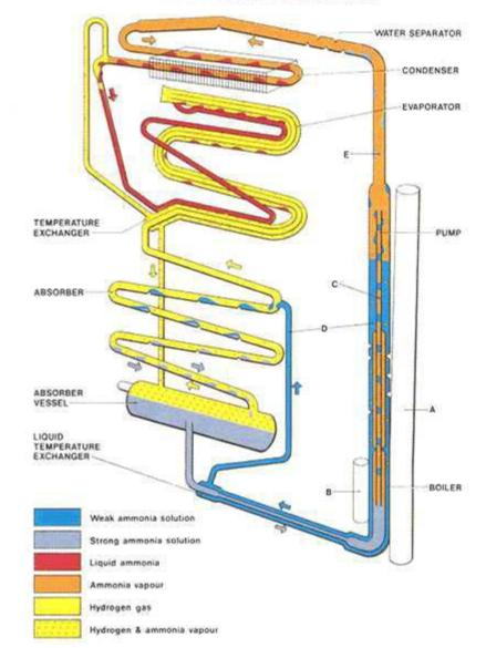
low-cost, noiseless, phase-change, absorption cooling technology was used extensively in "gas refrigerators", especially in urban-and-rural homes that had no electricity. Many modern designers are not familiar with the characteristics or economics of absorption cooling. It revived for use in Recreation vehicles.
