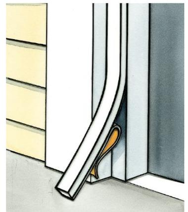
Use scissors to cut strip to fit, but don't remove backing paper yet.
