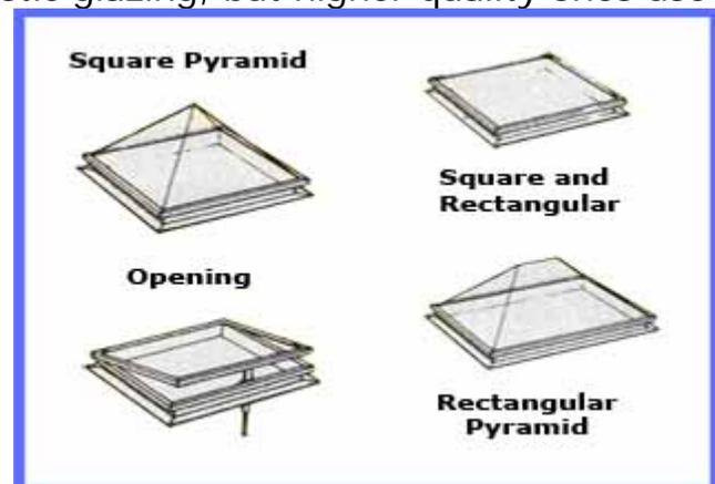
The slope or curvature of the glazing also helps to shed moisture and leaves. These skylight designs also do not require the additional framing needed to slope a flat skylight for proper drainage on flat or low-slope roofs.
