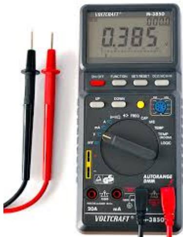
You're going to use this to test the cells power output. Once you connect the cells together you can check the voltage flow as you go. They should increase with each new cell connected. And measure your output once you've completed the panel. You can buy these cheap at Harbor freight tools, or even Wal-Mart.
