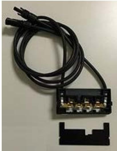
Most junction boxes will allow you to easily slide the bus wire from the solar panel inside the slot of the junction box. Once you slide the bus wires in, it is a good idea to solder the bus wires to the junction box leads.
