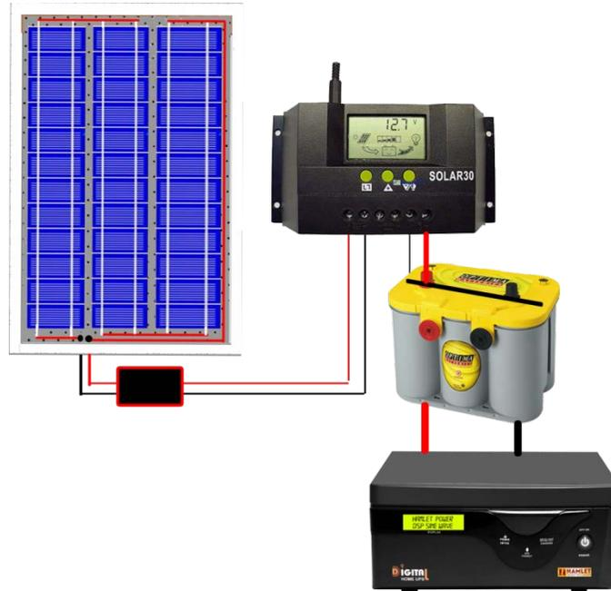
At this point, check the charge controller to make sure you're receiving solar energy. If it is, then hook your appliance into the inverter.
