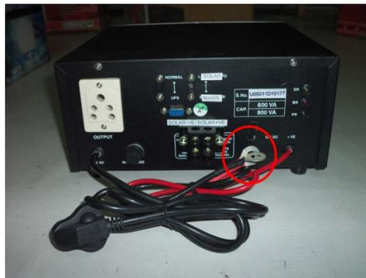
Roll out enough wire to connect the battery to the inverter. Connect the positive wire (Red) to the positive lead on the inverter. Connect the negative wire on the negative terminal.
